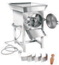
Pulverizer , T & T Cap.:2HP, 3HP, 5HP & 7HP
