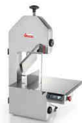
Bone Saws , Sirman Blade Length (mm): 1550, 1650 & 1840 Pulley: 210mm & 250mm
